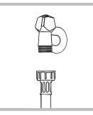
Connect the supply pipe by screwing it to a cold water tap using a 3/4 gas threaded connection (see figure).
